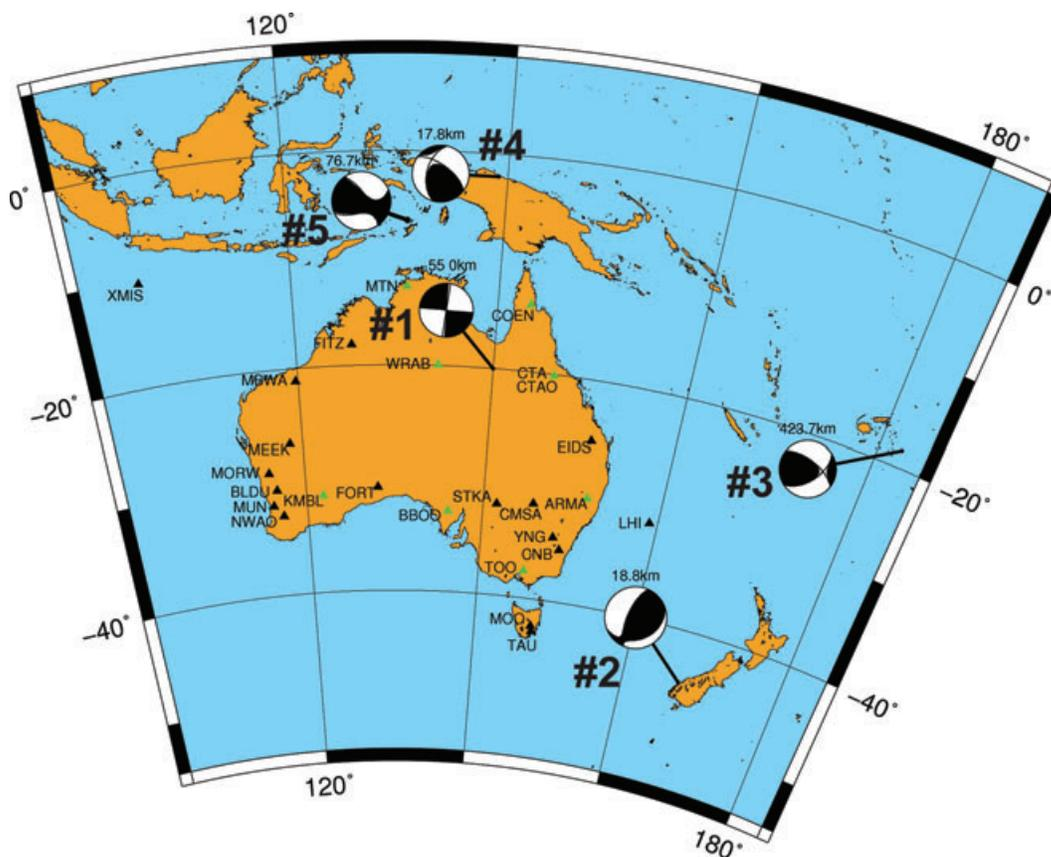
**Figure 2.** A map of Australasia, showing Australian permanent broadband seismic stations (triangles) and the five sources used in this study (lower-hemisphere projections displayed). Green triangles indicate stations used in the synthetic testing.
